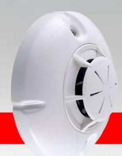
The fire detectors FD8010 and FD8020 provide reliable early warning of a fire condition upon ambient temperature reaching a fixed temperature threshold. They are available in two versions (A2S or BS for FD8010 and A2R or BR for FD8020) depending on the temperature threshold in accordance with the European Standard EN54-5.
